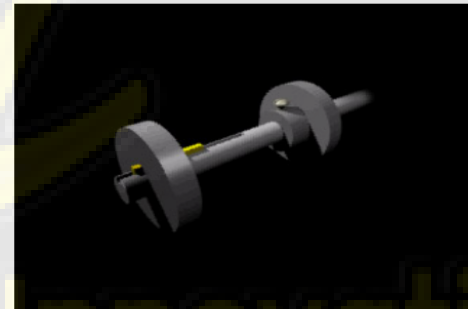
Rotating shaft and pulleys with projecting key and set screw
